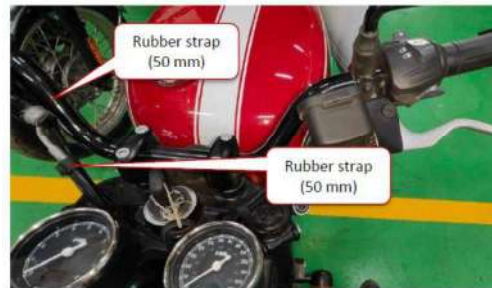
Control Sw. RH – • Brake sw. & control sw. cable to be strap with handlebar. • Wires to be strap together excluding throttle cable.
