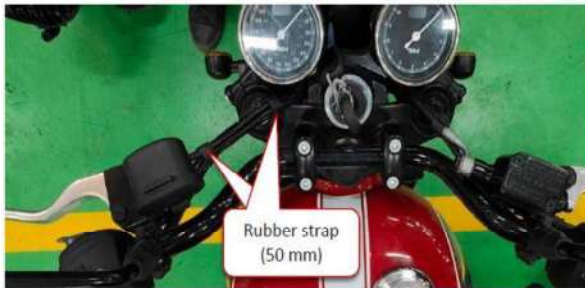
Control Sw. LH – Rubber strap to be used for wires excluding clutch cable.
