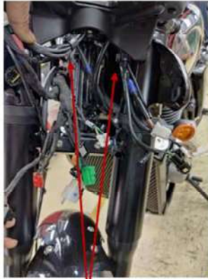
Wiring harness near head lamp area sort LH & RH side harness branches.
