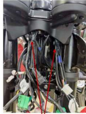
Wiring harness near head lamp area ( After condition). Assemble Rubber strap 60mm on LH as well as RH side.
