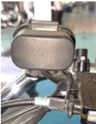
Control Sw. LH – Rubber strap to be used for wires excluding clutch cable.
